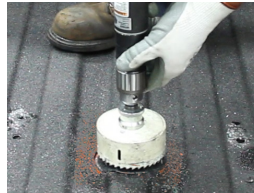
Use the pilot hole for error-free drilling
