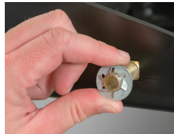
Retainer clips secure the bolts supporting the center section while attaching an installation kit
