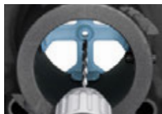
Simply drill up from under the bed
