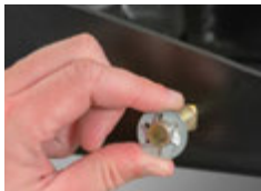
Retainer clips secure the bolts supporting the center section while attaching an installation kit
