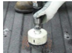
Use the pilot hole for error-free drilling
