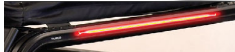
Rear Light bar works as a Secondary CHMSL
