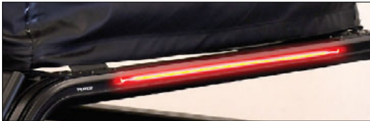
Rear light bar works as a secondary CHMSL
