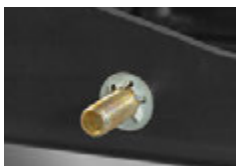
Retainer clips secure the bolts supporting the center section while attaching an installation kit
