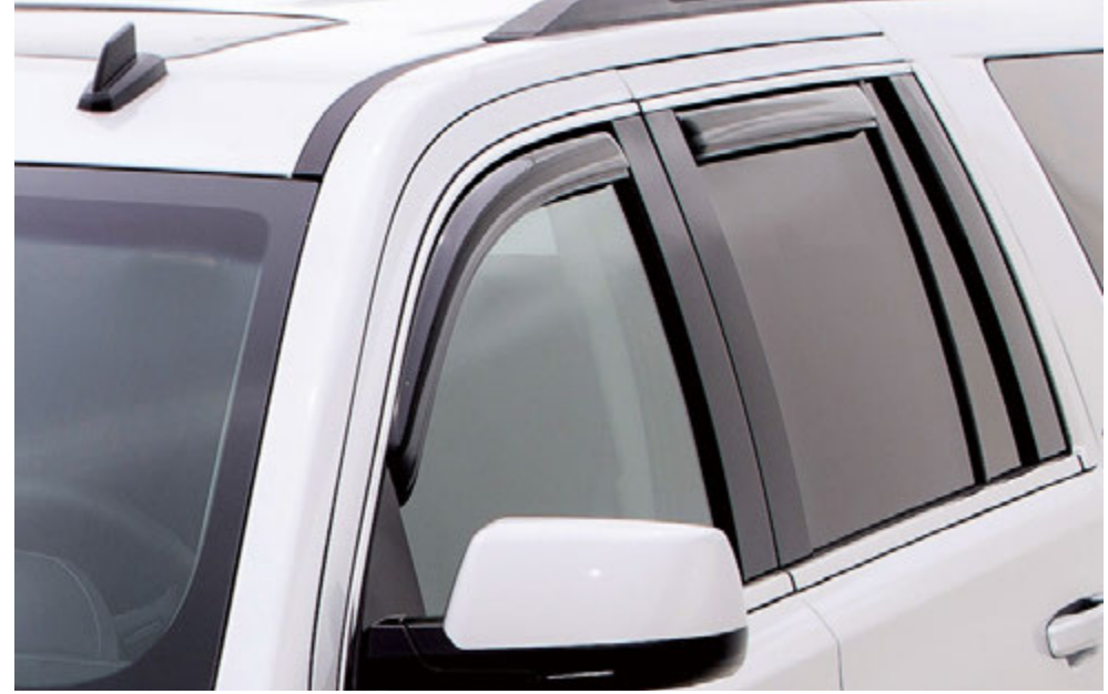
In-Channel Side Window Deflector in Smoke
