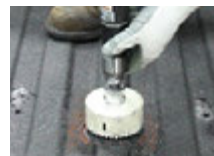
Use the pilot hole for error-free drilling
