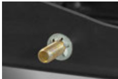
Retainer clips secure the bolts supporting the center section while attaching an installation kit
