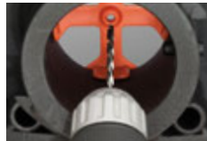
Simply drill up from under the bed
