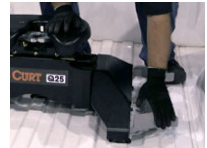
Close the anchor levers to lock the legs into place
