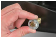
Retainer clips secure the bolts supporting the center section while attaching an installation kit
